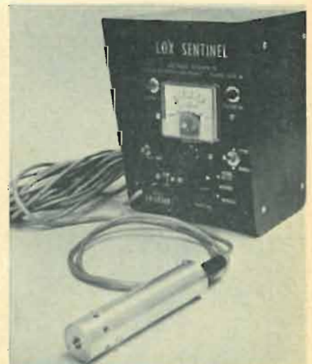
Capacitive probe senses presence of cryogenic fluids, sounds alarm, controls flow.
