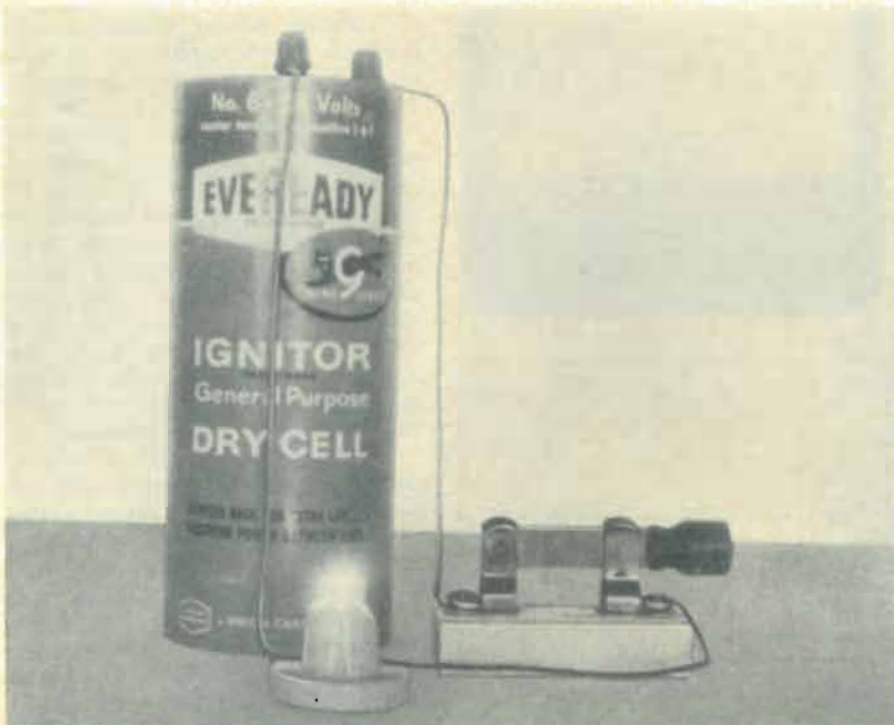
Simple circuit symbolizes basic principle of electric current flow between two points.
