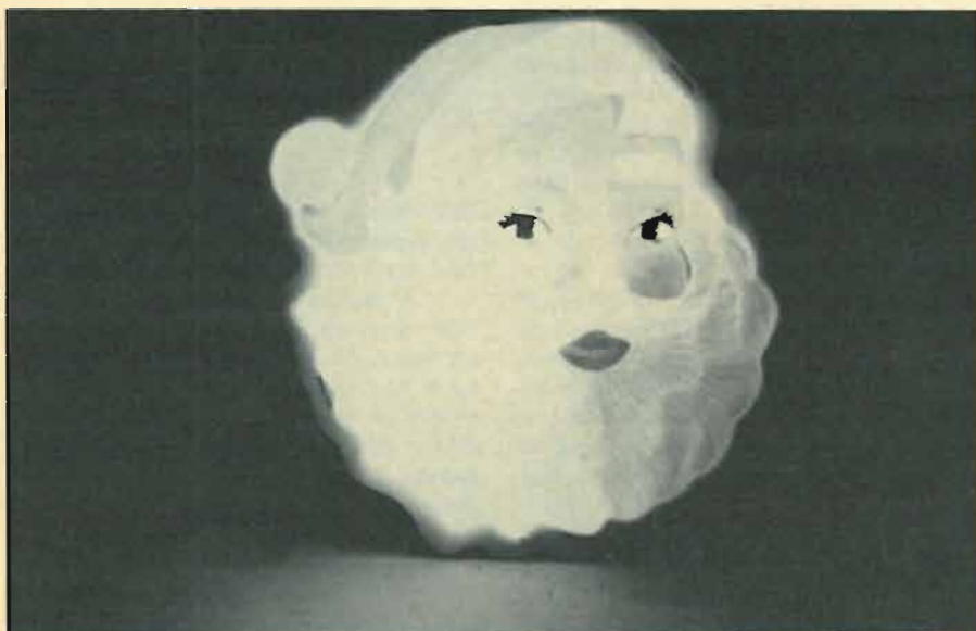
Santa's talking or singing is emphasized by variation in light intensity of display.
