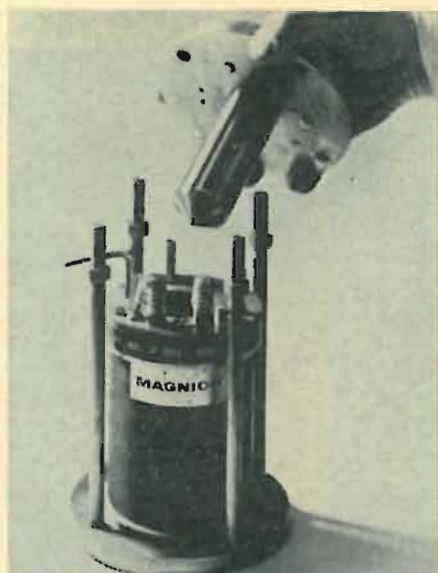
Magnet (top) becomes superconductive by immersion in liquid-helium tank (bottom).
