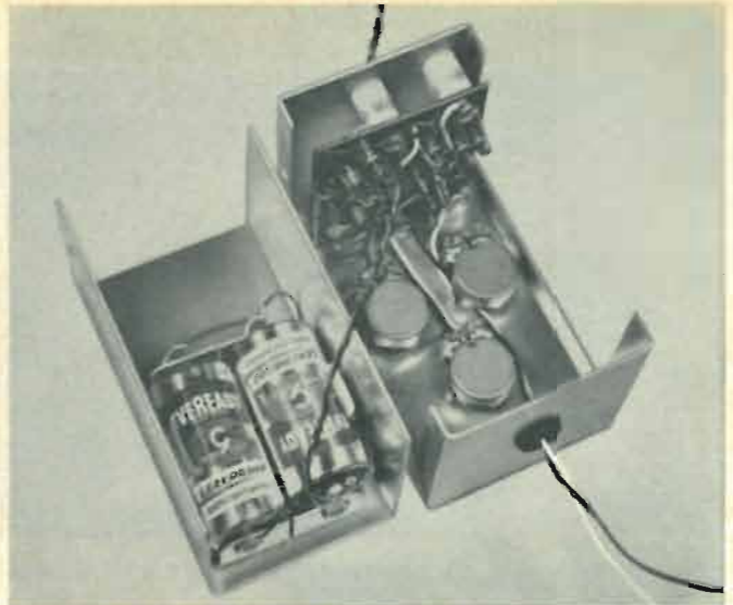
Perforated board, at top, can be used for easy mounting and wiring of components. Battery holder is attached to box lid.
