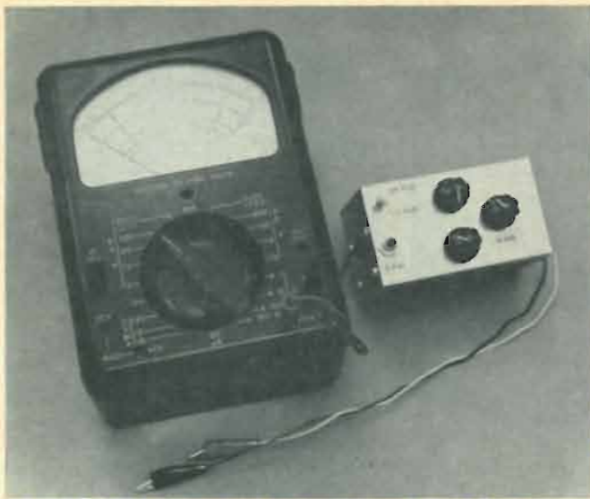
Output of high-impedance adapter connects to regular input of vom, while clip leads couple adapter input to measured circuit.
