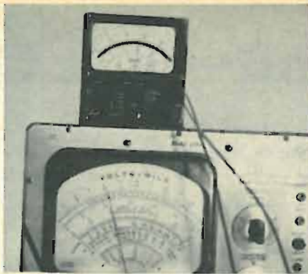
Why this difference in meter readings? The vom is isolated, but the vtvm isn't.
